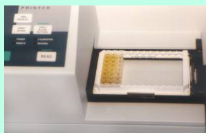
Read plates in a Plate Reader within 30 minutes of the addition of Stop Solution
